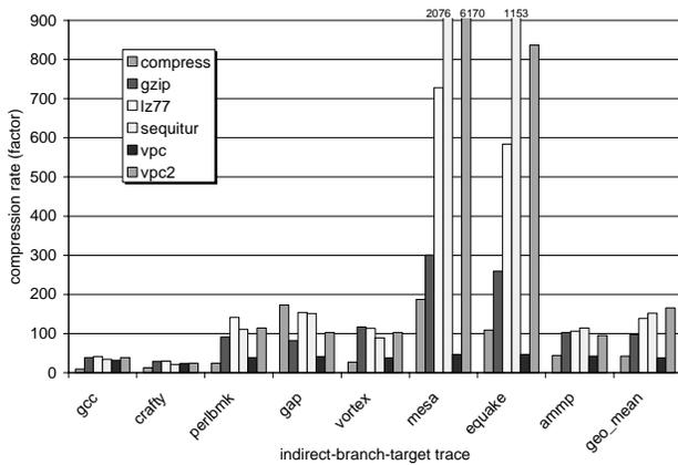
Figure 8: Compression rate on the indirect-branch-target traces.
