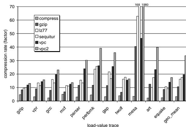
Figure 5: Compression rates on the load-value traces.
