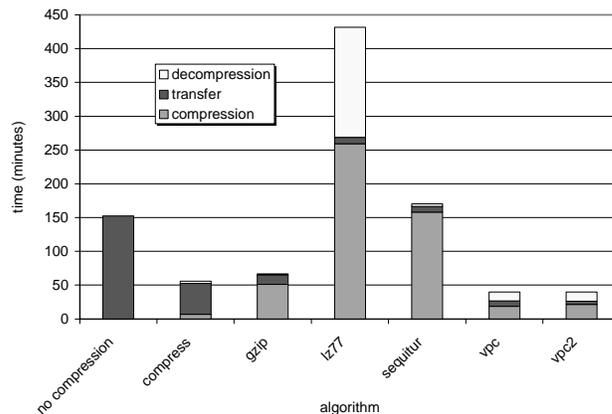
Figure 6: Average time to compress, send, and decompress a load-value trace.
