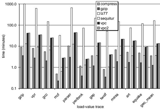
Figure 7: Decompression time on the load-value traces.
