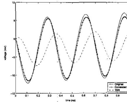
**Figure 3: Simulation results for one output on RC network example. PMTBR with correlation information out-performs TBR.**
