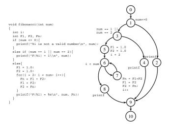
Fig. 1. C code for the Fibonacci program and its CDFG.
