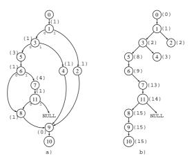
Fig. 2. DAG of Fibonacci example and corresponding tree. **PROGRAM DAG**
