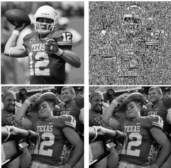
Fig. 5. Upper images are produced by a conventional IDCT with scaled V_{DD} . Techniques of [63] improve image quality for the same scaled V_{DD} in the lower images.
